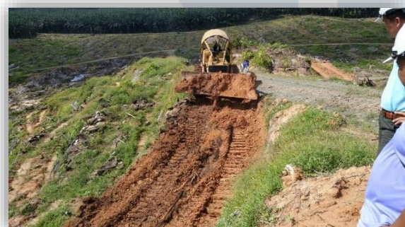
Machines were used during the replanting exercise to carry out trunk chipping (left) and terracing (right)
